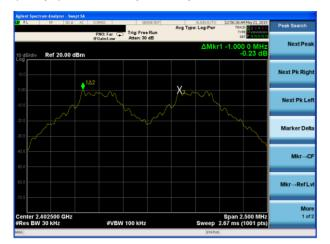
(2Mbps) Channel Separation plot on channel 00-01
