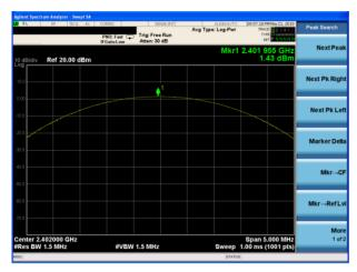
Peak output Power plot on channel 39 (3Mbps)
