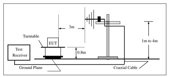
(c) For radiated emissions above 1000MHz
