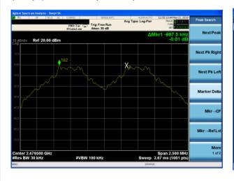
(2Mbps) Channel Separation plot on channel 77-78
