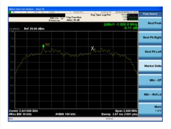
(3Mbps) Channel Separation plot on channel 77-78
