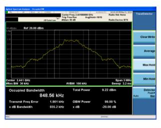
20dB Bandwidth plot on channel 39 (2Mbps)
