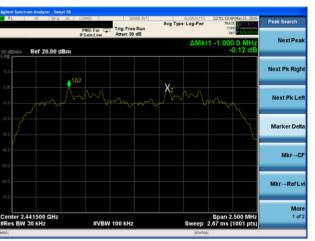
(1Mbps) Channel Separation plot on channel 77-78
