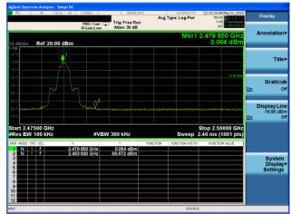
π /4-DQPSK: Band Edge-High Channel (Hopping Mode)
