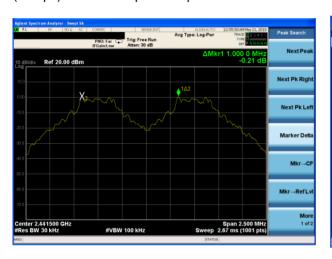
(2Mbps) Channel Separation plot on channel 39-40
