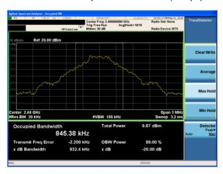
20dB Bandwidth plot on channel 78 (2Mbps)
