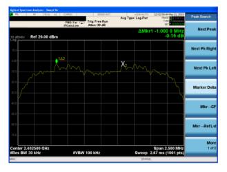
(3Mbps) Channel Separation plot on channel 39-40
