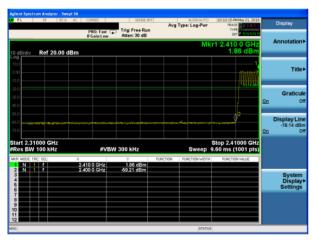
GFSK: Band Edge-High Channel (Hopping Mode)
