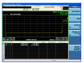
8-DPSK: Band Edge-High Channel (Hopping Mode)
