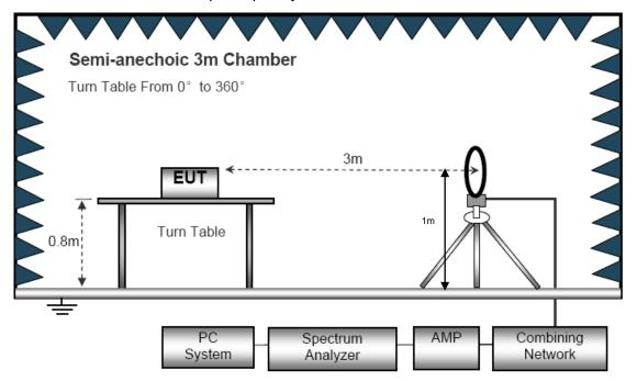
(B) Radiated Emission Test-Up Frequency 30MHz~1GHz
