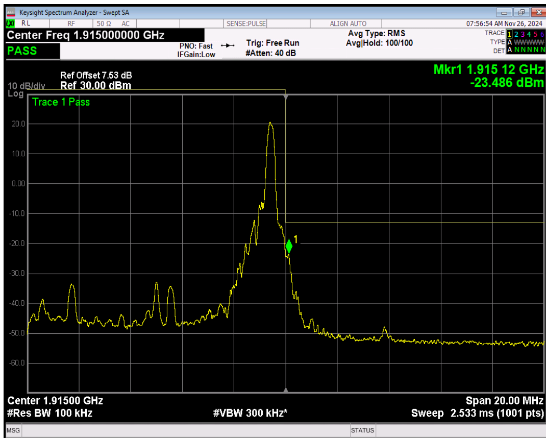
Band25 16QAM BW=10MHz Channel=26640 RB Size=50 Position=#0
