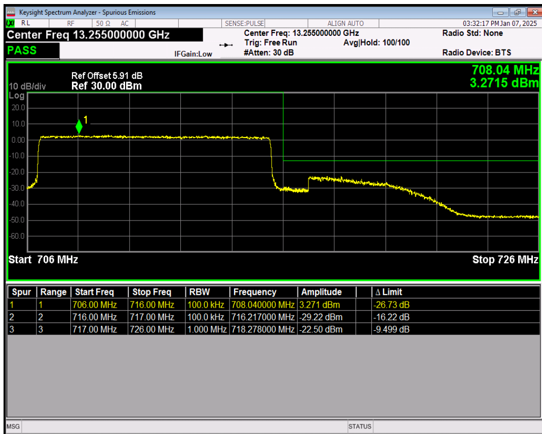
Band2 QPSK BW=3MHz Channel=19185 RB Size=1 Position=#Max
