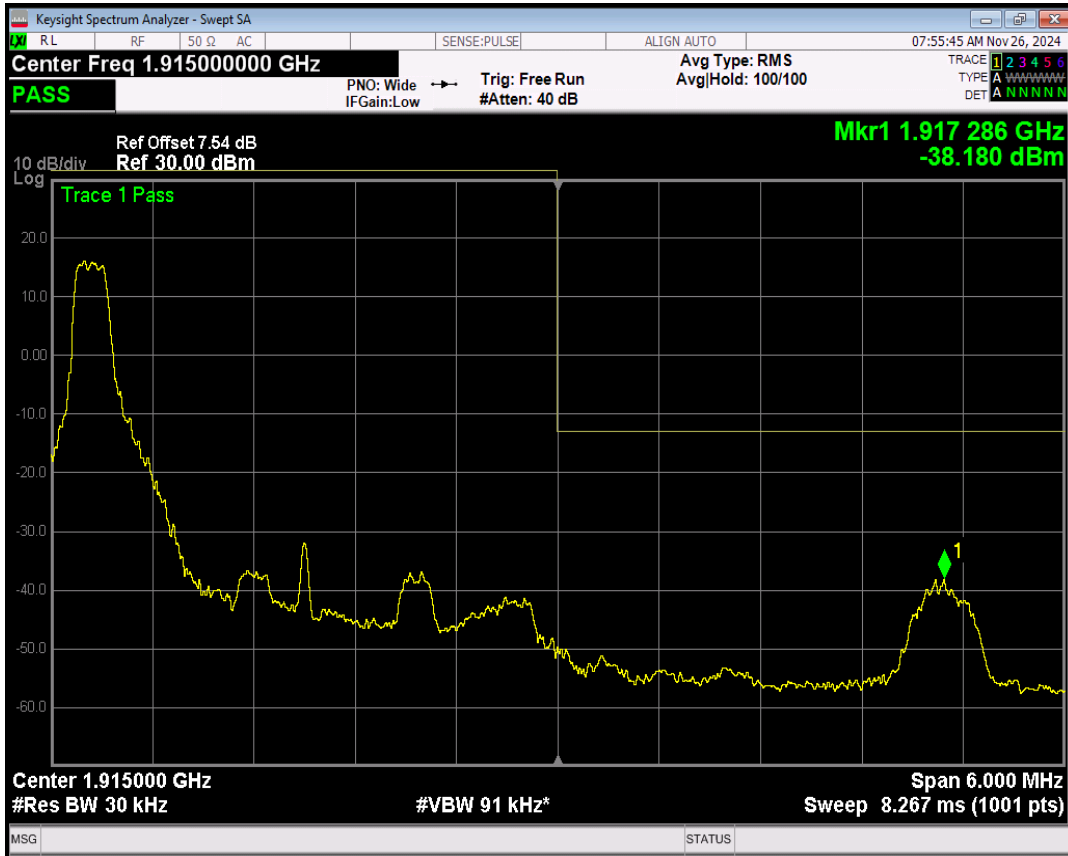
Band25 16QAM BW=3MHz Channel=26675 RB Size=1 Position=#Max
