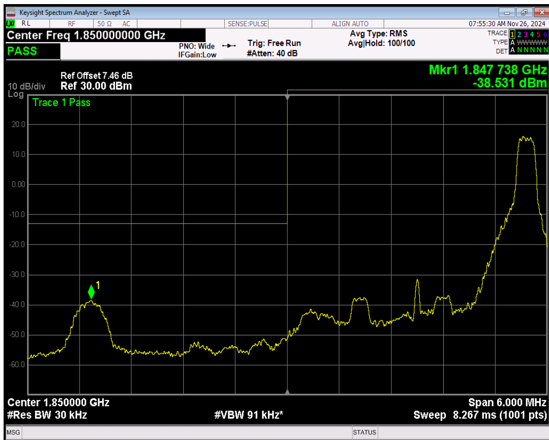
Band25 16QAM BW=3MHz Channel=26055 RB Size=15 Position=#0
