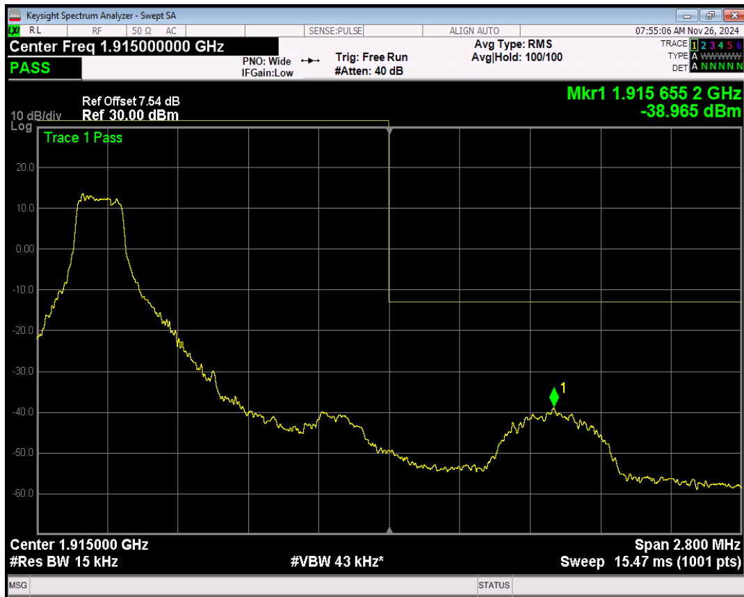
Band25 16QAM BW=1.4MHz Channel=26683 RB Size=1 Position=#Max
