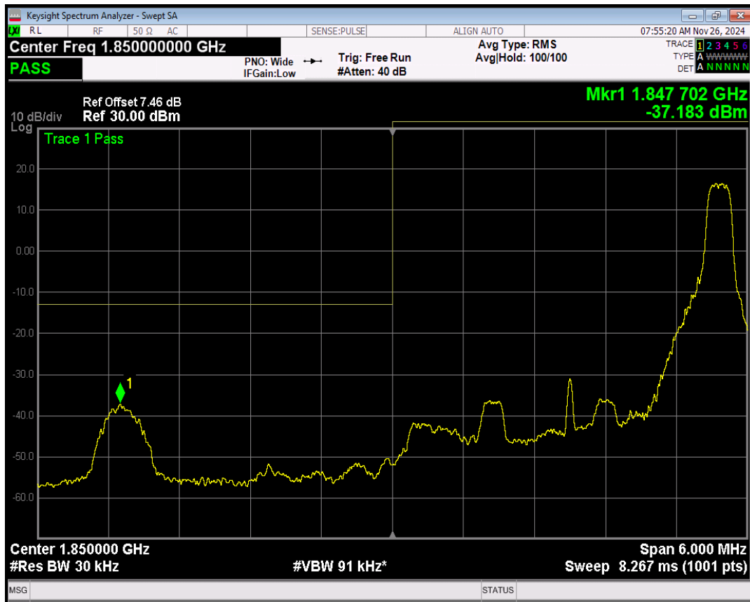
Band25 QPSK BW=3MHz Channel=26055 RB Size=15 Position=#0
