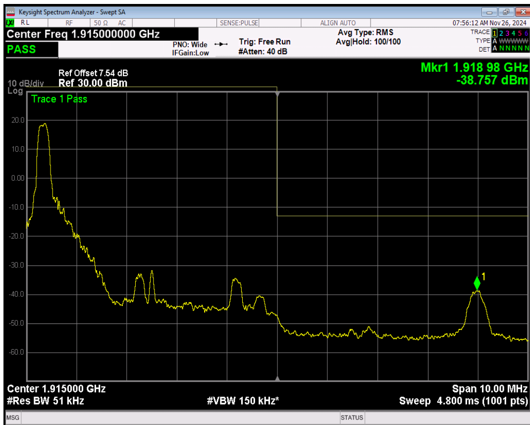
Band25 QPSK BW=5MHz Channel=26665 RB Size=1 Position=#Max
