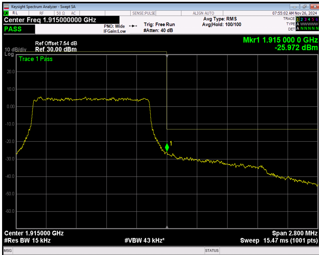
Band25 16QAM BW=1.4MHz Channel=26683 RB Size=1 Position=#0
