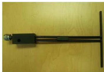
Figure 1 – MVG COMOSAR Validation Dipole
