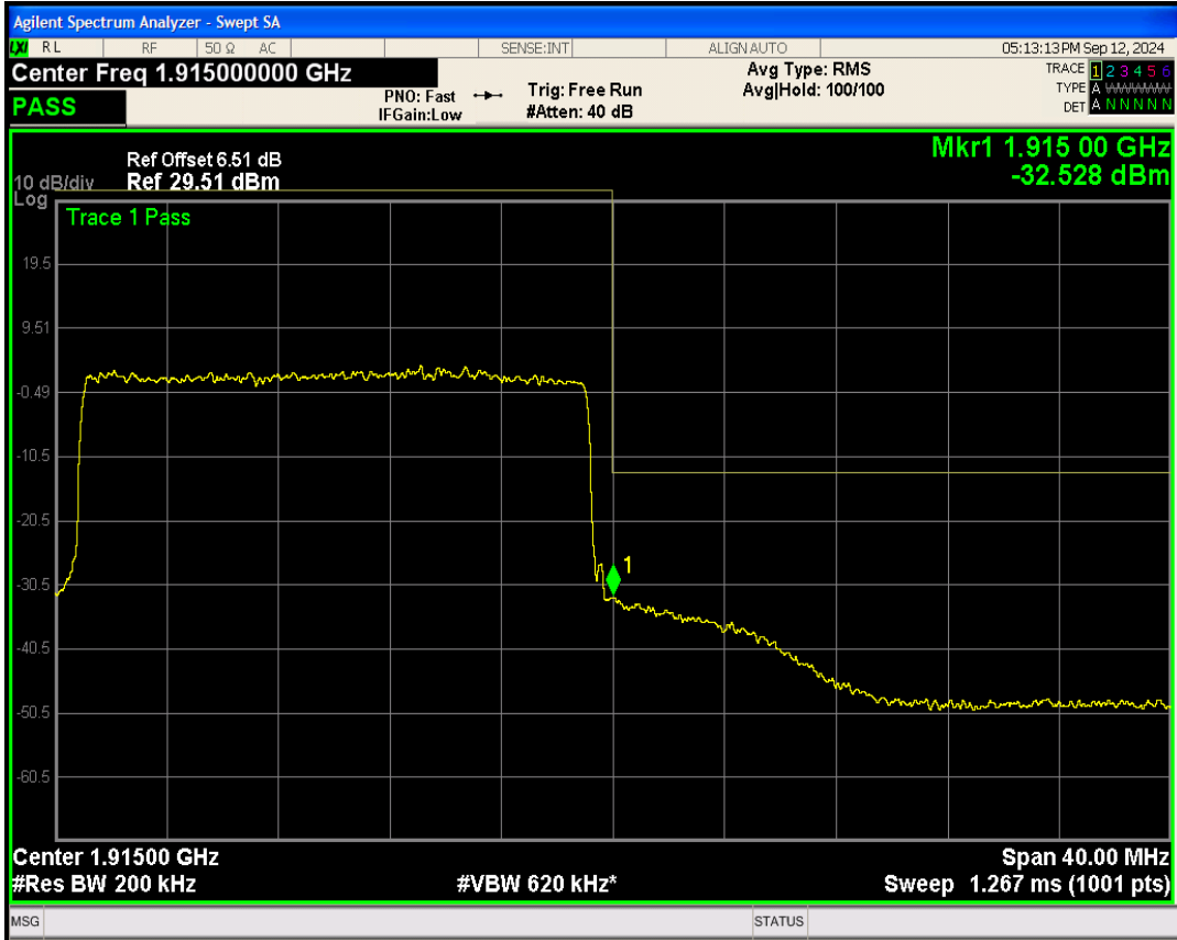
Band25 16QAM BW=20MHz Channel=26590 RB Size=100 Position=#0
