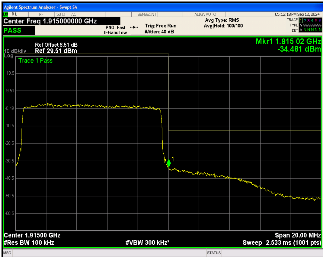
Band25 QPSK BW=15MHz Channel=26115 RB Size=75 Position=#0
