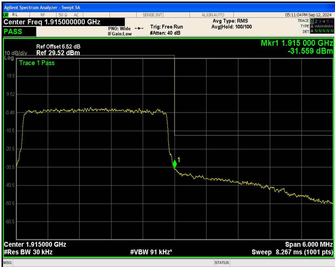
Band25 QPSK BW=5MHz Channel=26065 RB Size=25 Position=#0
