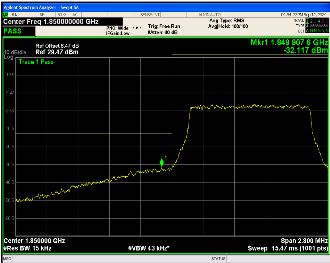
Band25 QPSK BW=1.4MHz Channel=26683 RB Size=6 Position=#0
