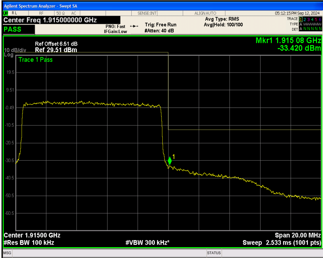
Band25 16QAM BW=10MHz Channel=26640 RB Size=50 Position=#0
