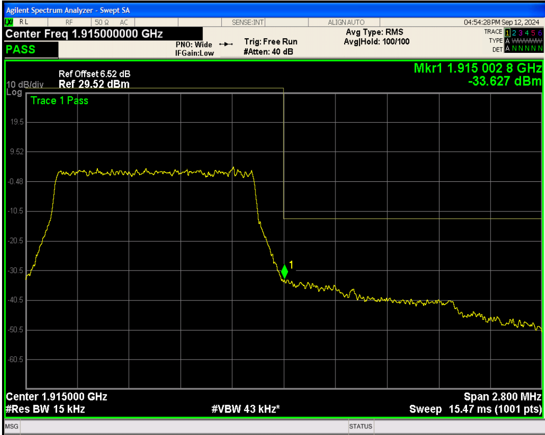
Band25 16QAM BW=1.4MHz Channel=26683 RB Size=6 Position=#0
