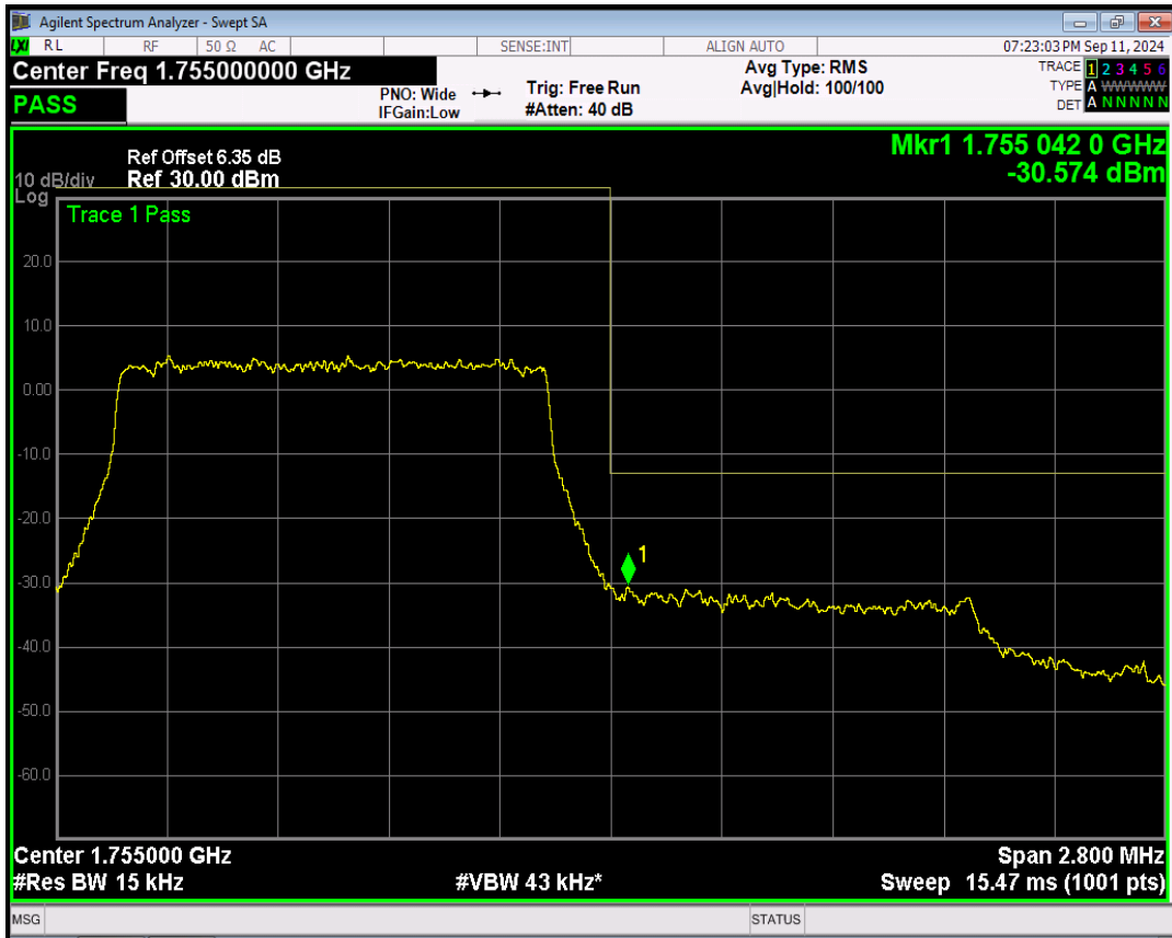
Band4 16QAM BW=1.4MHz Channel=20393 RB Size=6 Position=#0
