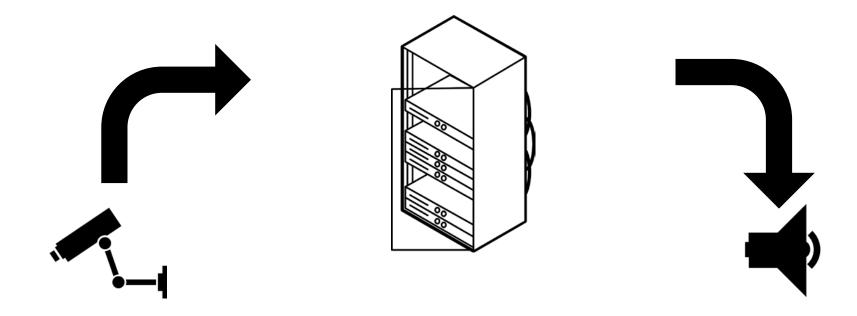
When another device signals the server, it receives data from the server and rings the bell.
