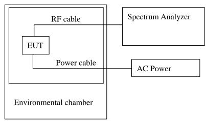
Note1: The frequency stability is measured with the temperature variation range of 0°C to +60°C (10°C increment), and voltage supply variation range of 90% to 110% of nominal DC supply voltage.
