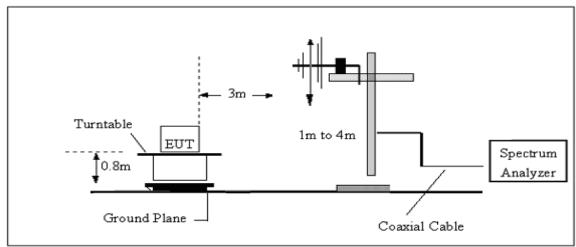
3. Radiated Emission Test-Up Frequency Above 1GHz
