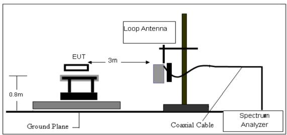
2. Radiated Emission Test-Up Frequency 30MHz~1GHz
