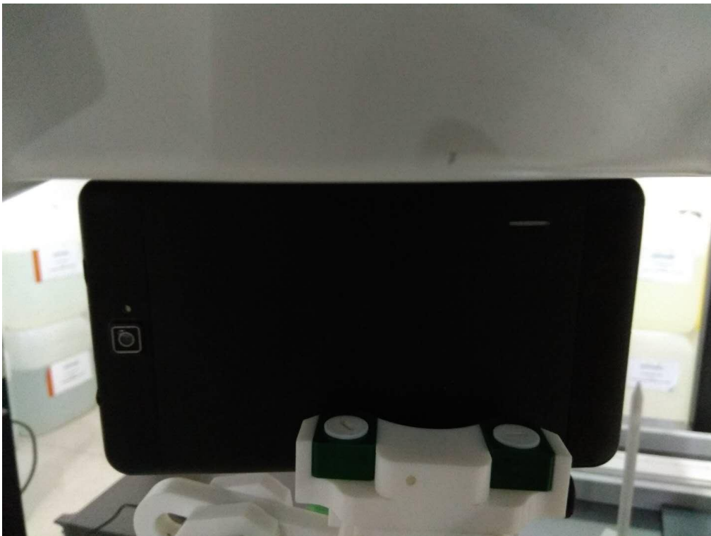
Body left side(separation distance is 0mm)
