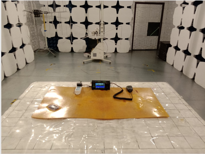
Photograph of test setup for Radiated disturbance
