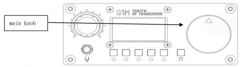
The five multi-function buttons at the bottom of the screen correspond to the displayed function menu.
