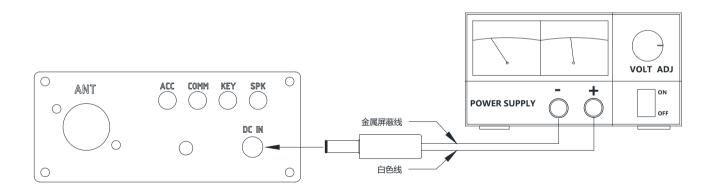
When the G1M uses an external power supply, in order to prevent external interference from entering the radio through the power line, and radio frequency interference in the radio radiates outward through the power line, an EMC magnetic ring can be placed on the power line. Install the magnetic ring as close as possible to the side of the power plug.
