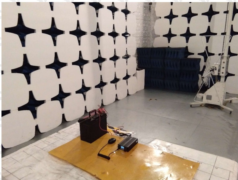
Photograph of test setup for Radiated disturbance
