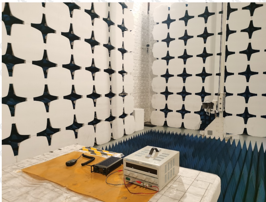
Photograph of test setup for Radiated disturbance
