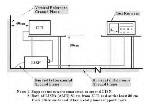
The measurement procedure of EUT setup is according with ANSI C63.10-2013. The related limit was specified in FCC Part 15.207.
