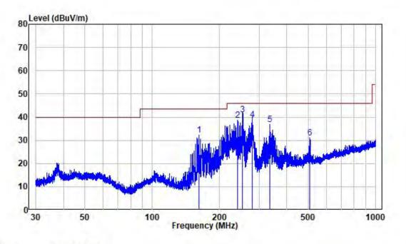
Site : chamber Condition: 3m HORIZONTAL Job No. : SZ4220608-25174E-RF Test Mode: USB 0.55MHz
