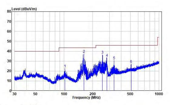
Site : chamber Condition: 3m VERTICAL Job No. : SZ4220608-25174E-RF Test Mode: AM 15.275MHz
