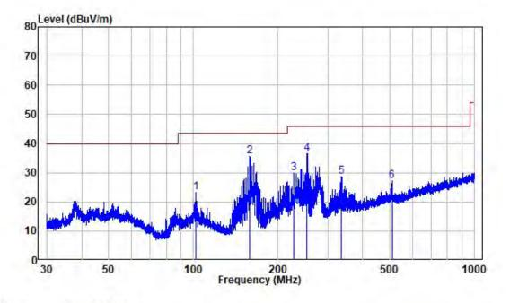
Site : chamber Condition: 3m VERTICAL Job No. : SZ4220608-25174E-RF Test Mode: CW 15.275MHz
