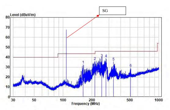
Site : chamber Condition: 3m HORIZONTAL Job No. : SZ4220608-25174E-RF Test Mode: FM 108MHz
