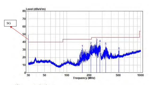
Site : chamber Condition: 3m HORIZONTAL Job No. : SZ4220608-25174E-RF Test Mode: USB 30MHz
