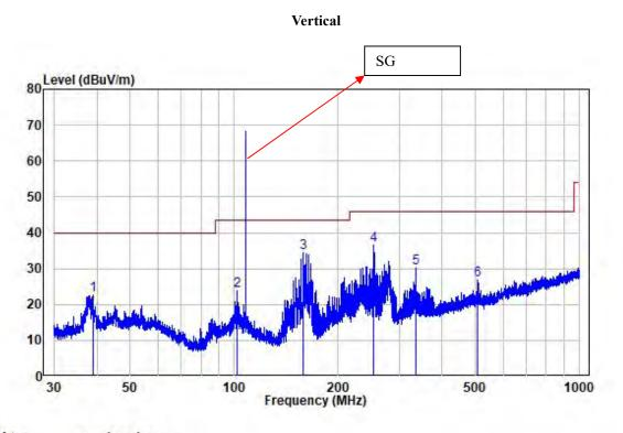
Site : chamber Condition: 3m VERTICAL Job No. : SZ4220608-25174E-RF Test Mode: FM 108MHz
