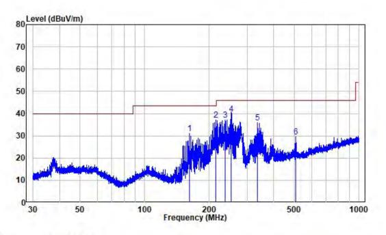
Site : chamber Condition: 3m HORIZONTAL Job No. : SZ4220608-25174E-RF Test Mode: USB 15.275MHz
