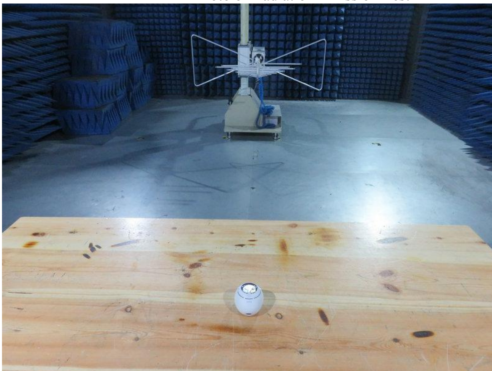
Photo of Radiation Emission Test
