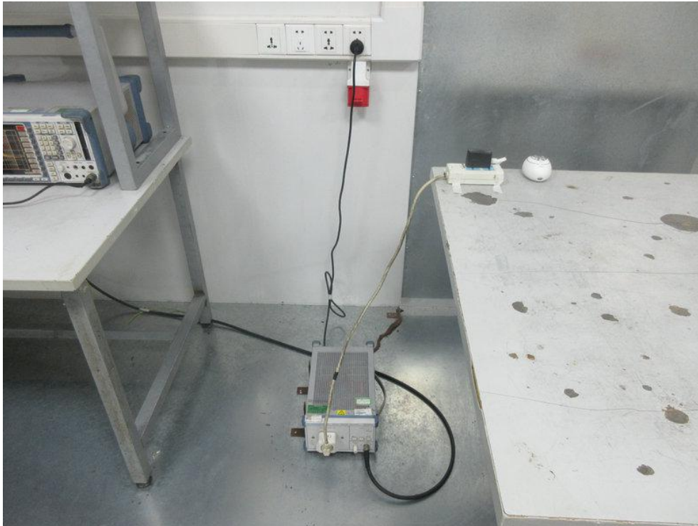
Photo of Power Line Conducted Emission Test
