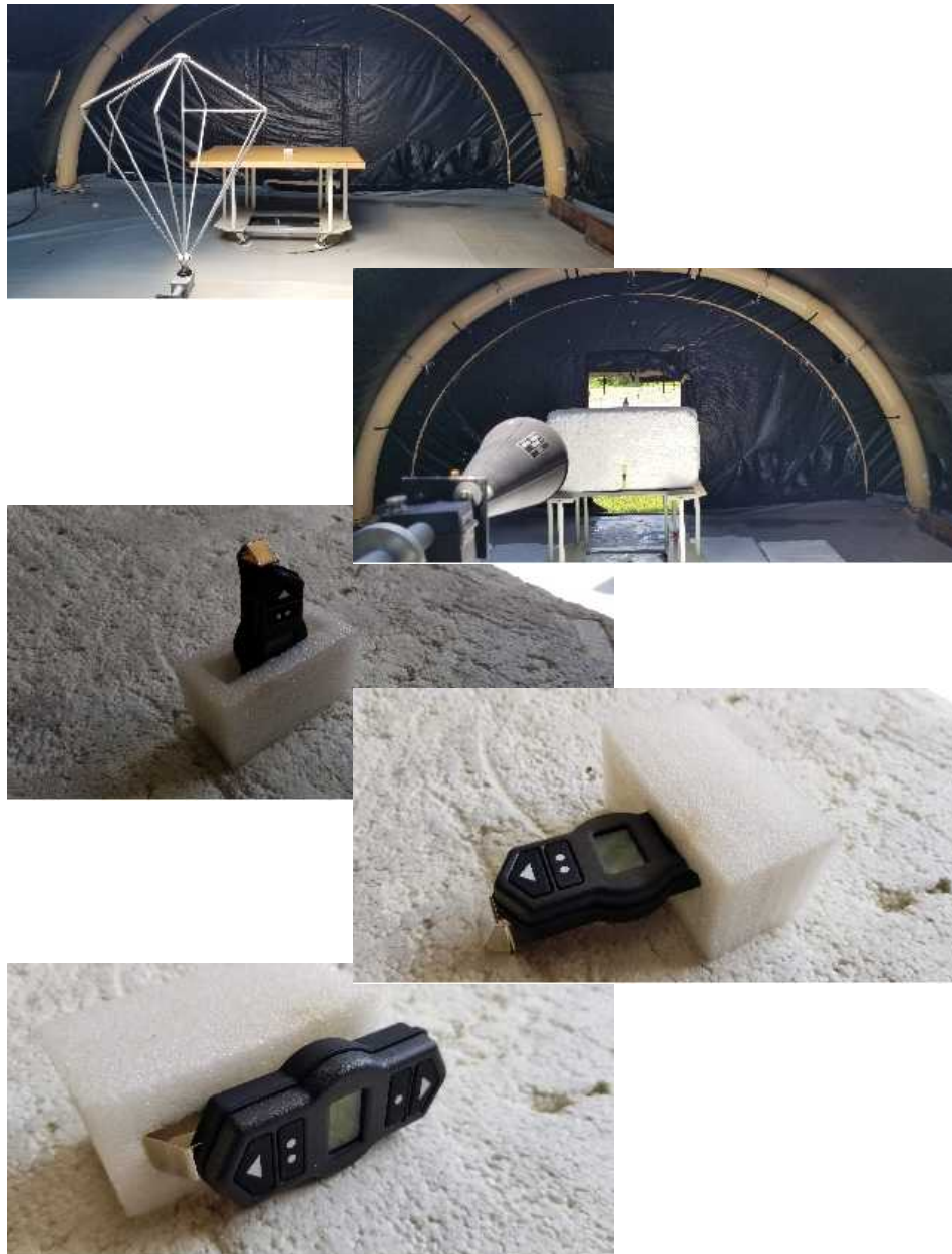
Figure 4: Radiated Emissions Test Setup Photograph(s).
