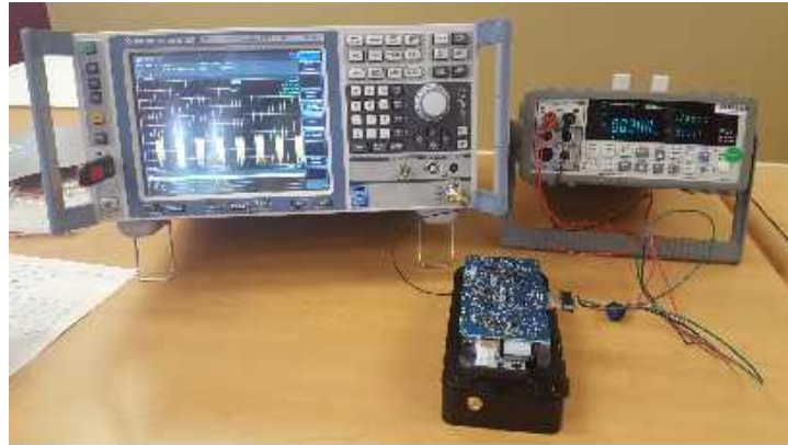
Figure 5: Conducted RF Test Setup Photograph(s).
