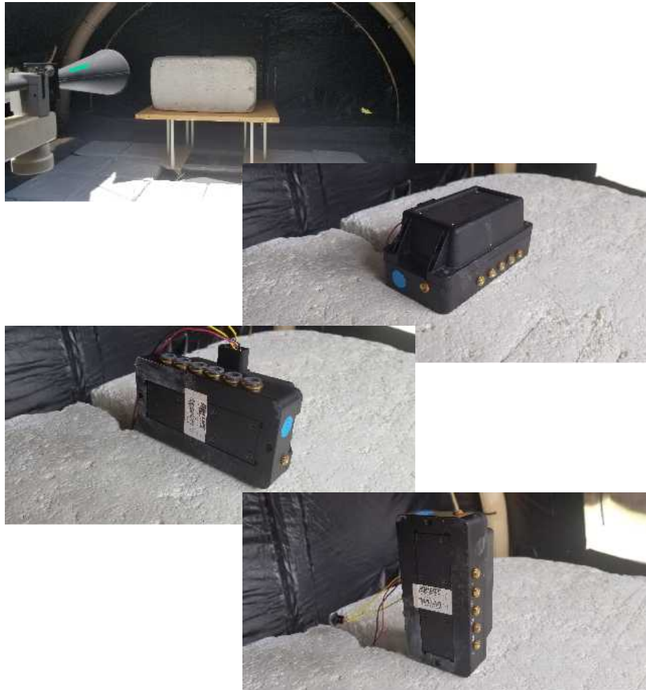
Figure 4: Radiated Emissions Test Setup Photograph(s).
