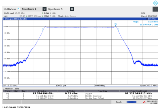
Figure 8.1-15: 99% OBW Middle channel: 15.55 GHz, shortest pulse (100 MHz BW)
