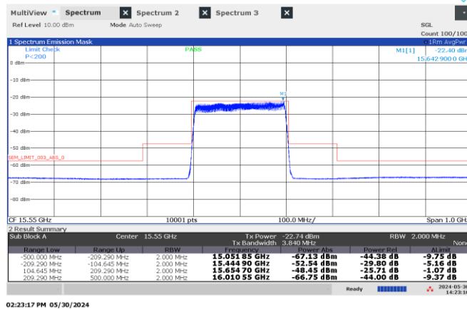
Figure 8.4-47: Emission mask, Middle channel: 15.55 GHz, shortest pulse. (200 MHz BW)
