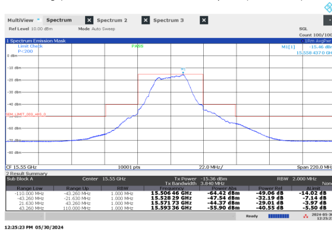
Figure 8.4-29: Emission mask, Middle channel: 15.55 GHz, shortest pulse. (25 MHz BW). RBW/2 Added at the edges.
