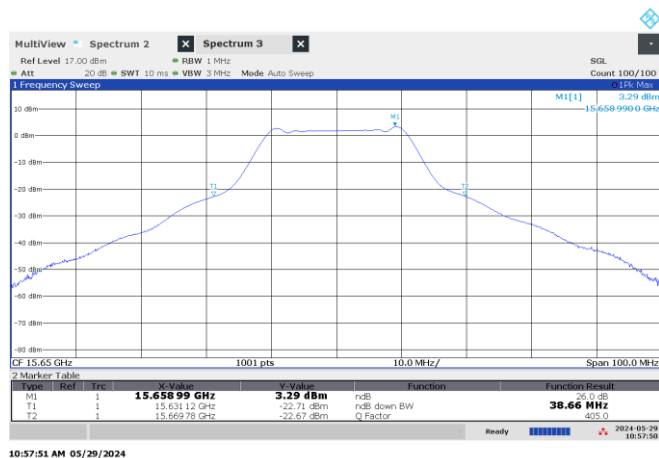
Figure 8.2-11: 26 dB OBW High channel: 15.65 GHz, shortest pulse (25 MHz BW)
