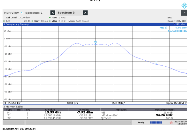
Figure 8.2-13: 26 dB OBW Middle channel: 15.55 GHz, shortest pulse (50 MHz BW)
