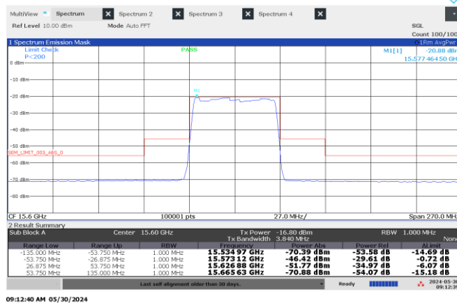
Figure 8.4-17: Emission mask, High channel: 15.60 GHz, longest pulse. (50 MHz BW)
