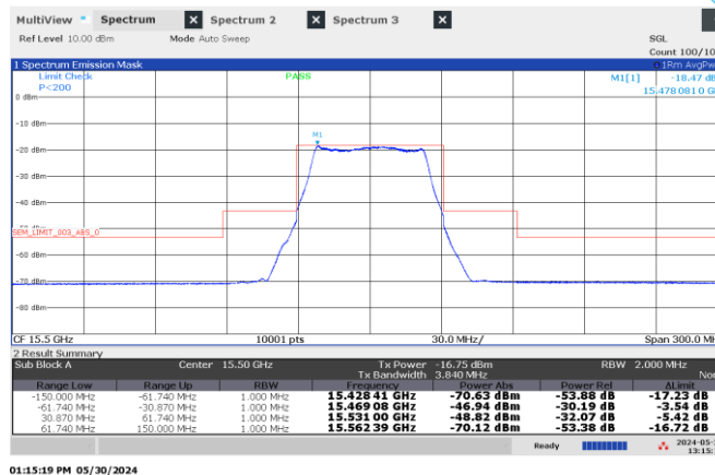
Figure 8.4-35: Emission mask, Low channel: 15.50 GHz, shortest pulse. (50 MHz BW)
