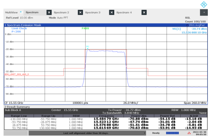
Figure 8.4-14: Emission mask, Middle channel: 15.55 GHz, longest pulse. (50 MHz BW)
