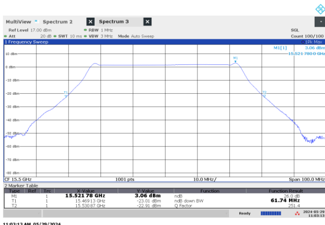
Figure 8.2-12: 26 dB OBW Low channel: 15.50 GHz, shortest pulse (50 MHz BW)
