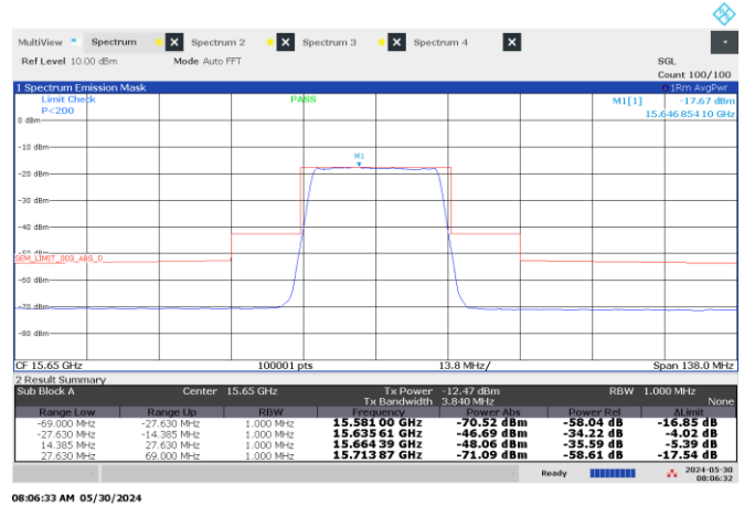
Figure 8.4-8: Emission mask, High channel: 15.65 GHz, longest pulse. (25 MHz BW)
