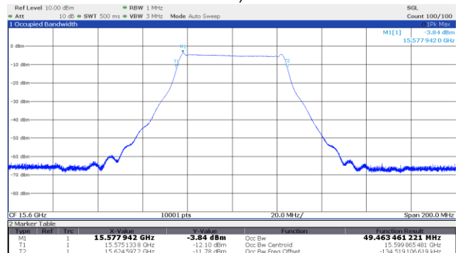
Figure 8.1-14: 99% OBW High channel: 15.60 GHz, shortest pulse (50 MHz BW)
