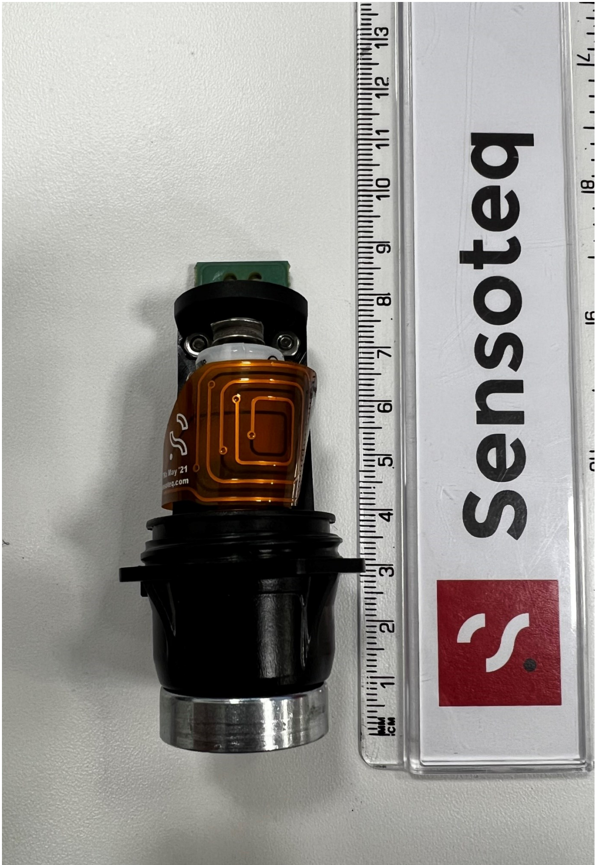
PCB with Base including battery rear
