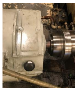
Sensor Mounted on Bearing Housing
