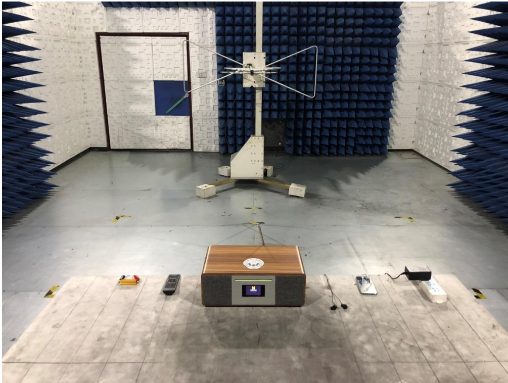
FCC RADIATED EMISSION TEST SETUP ABOVE 1GHZ
