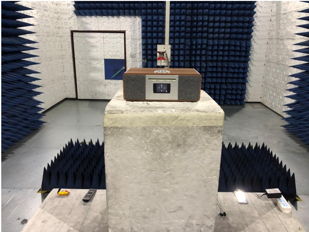
FCC RADIATED EMISSION TEST SETUP ABOVE 1GHZ
