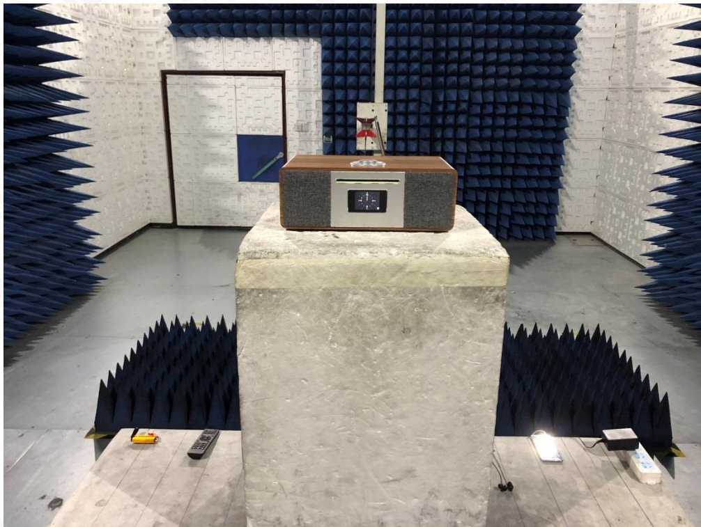
FCC RADIATED EMISSION TEST SETUP ABOVE 1GHZ
