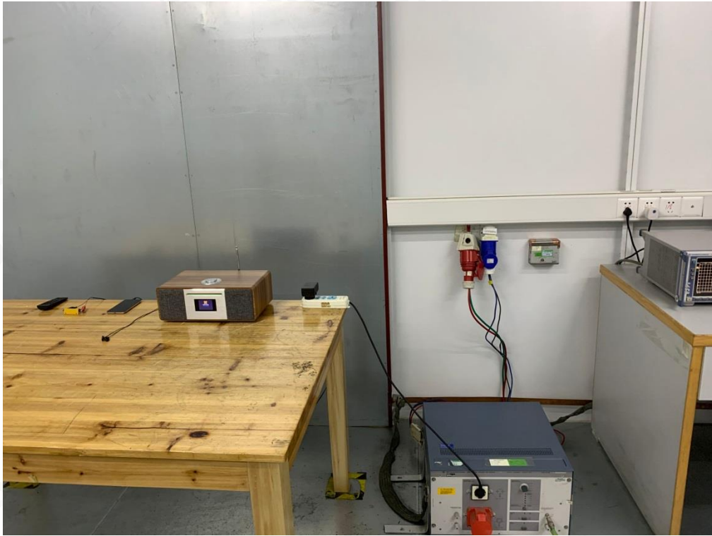
CONDUCTED TEST SETUP
