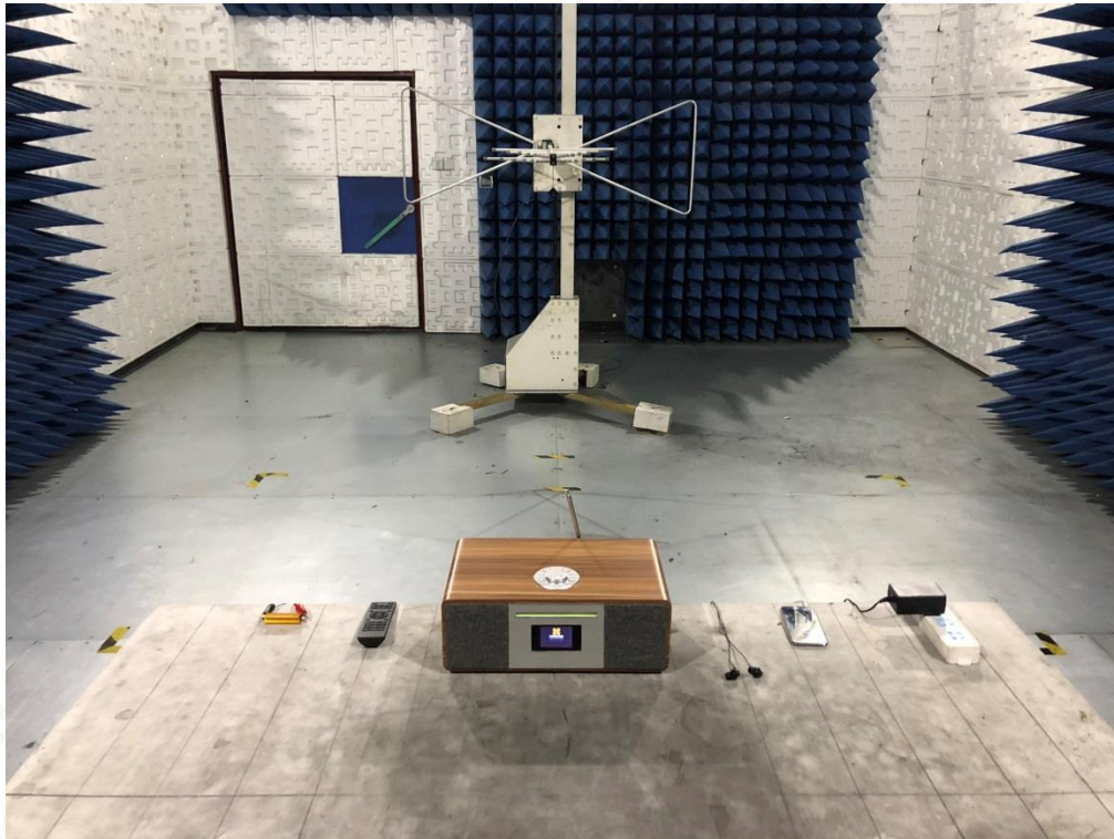
FCC RADIATED EMISSION TEST SETUP ABOVE 1GHZ
