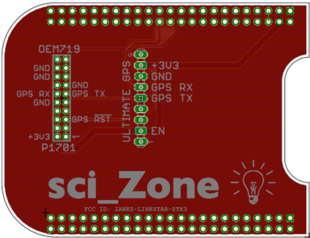
The FCC ID will also be permanently labeled onto the LinkStar-STX3 PC board (**SZ-LS-CAPE-100001**), 8 point font:
