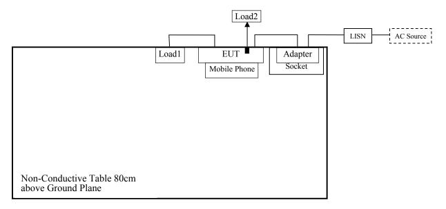
For Radiated Emissions (Below & Above 30MHz):
