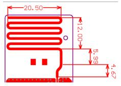
Antenna transmission frequency: 433.92MHz Antenna type: PCB antenna Antenna Gain: -10.098 dBi
