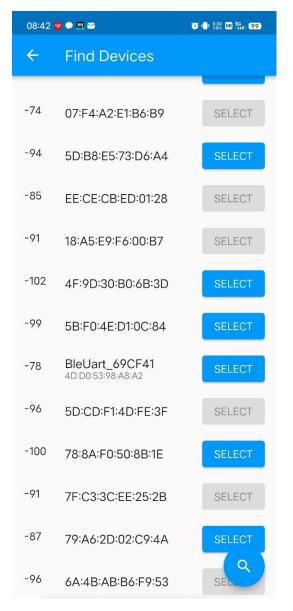
2) Find the device starting with BleUart, that is our Bluetooth box device, click SELECT to pop up the pairing interface, click OK twice to connect.
