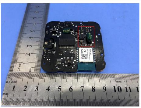
The new PCB delete the audio noise reduction IC module(AC107).
