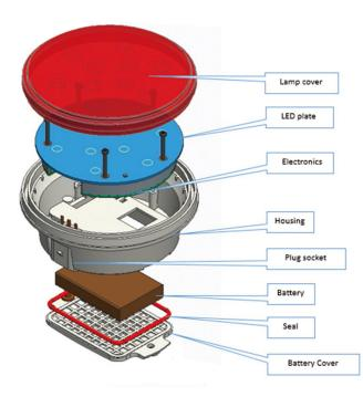
It looks and functions exactly the same as a standard 4" LED tail lamp, providing the ultimate in covert tracking and simple installation. Designed to function in the harsh conditions on the road, it is waterproof and shock proof.
