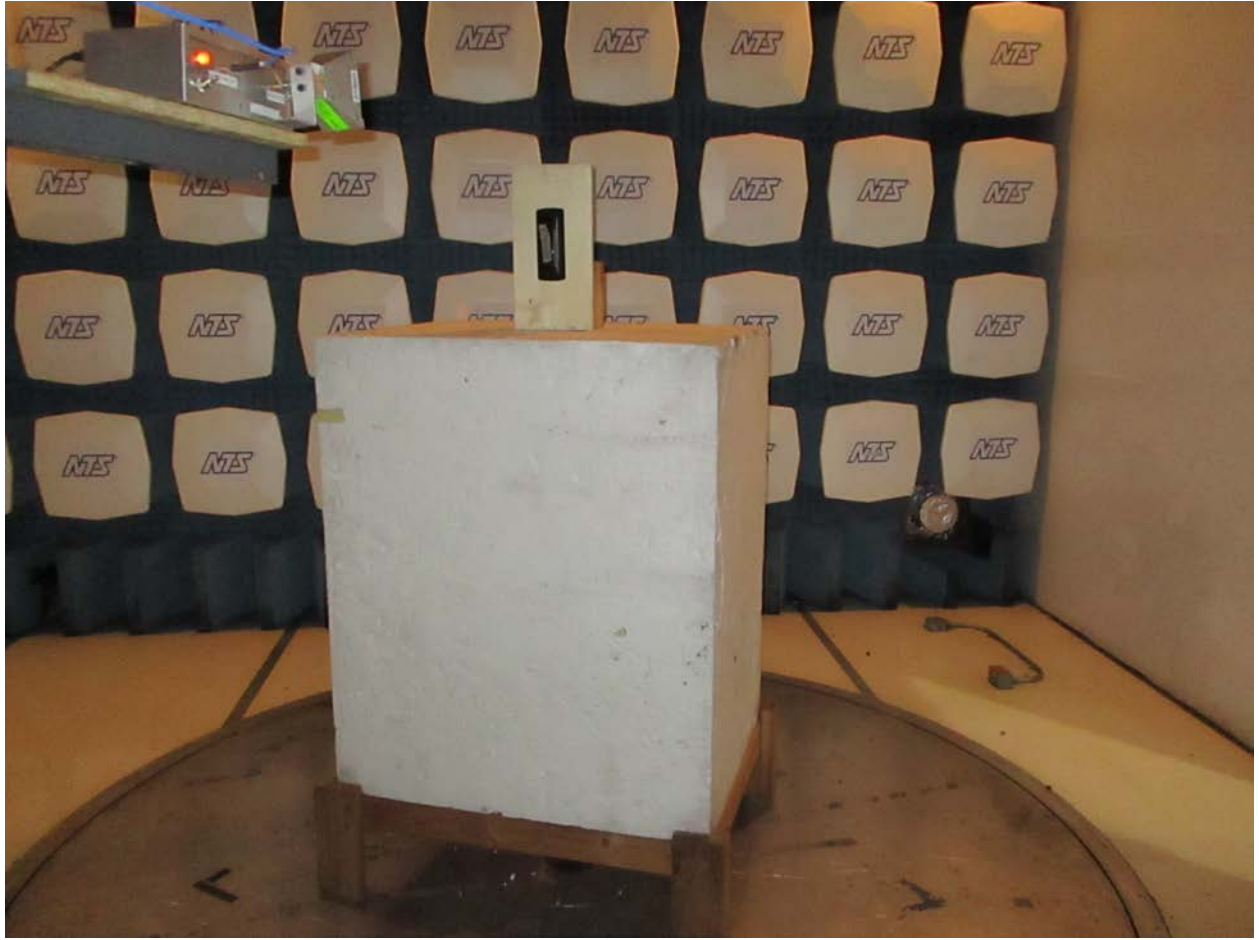
Radiated Measurements Setup 18-25GHz
