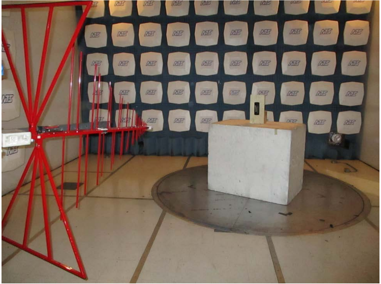
Radiated Measurements Setup 30-1000MHz
