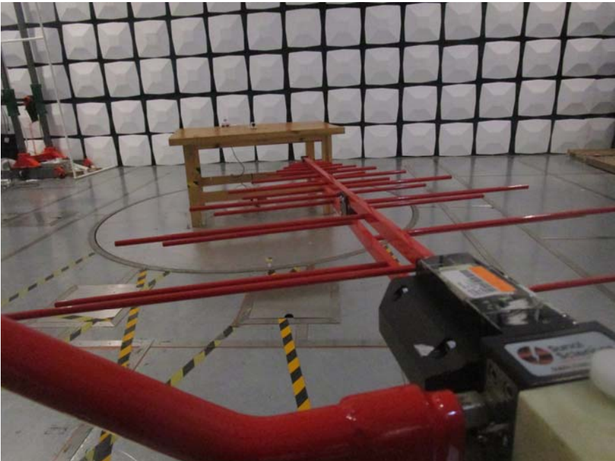
Radiated Emission Below 1GHz View
