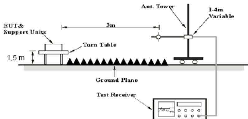
The radiated emission tests were performed in the 3 meters chamber test site A for the range 30MHz to 1GHz and the 3 meters chamber B test site for above 1GHz, using the setup accordance with the ANSI C63.10-2013. The specification used was the FCC 15.209, and FCC 15.247, the RSS-247 §5.5,RSS-Gen §8.10 limits..
