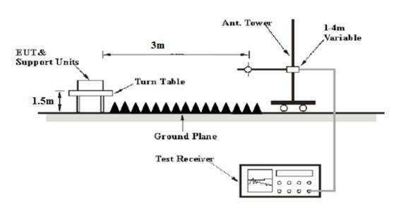
The radiated emission below 1GHz tests were performed in the 3 meters chamber test site A, above 1GHz tests were performed in the 3 meters chamber test site B, using the setup accordance with the ANSI C63.10-2013. The specification used was the FCC 15.209, and FCC 15.249 limits.
