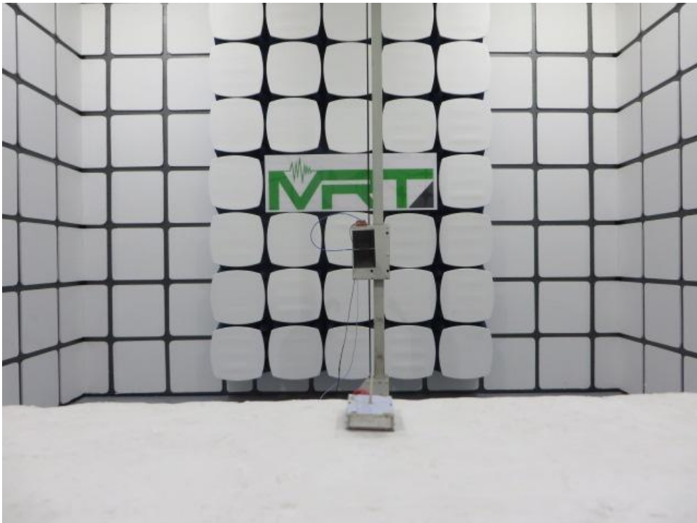
Description: Radiated Emissions Test Setup for Above 1GHz
