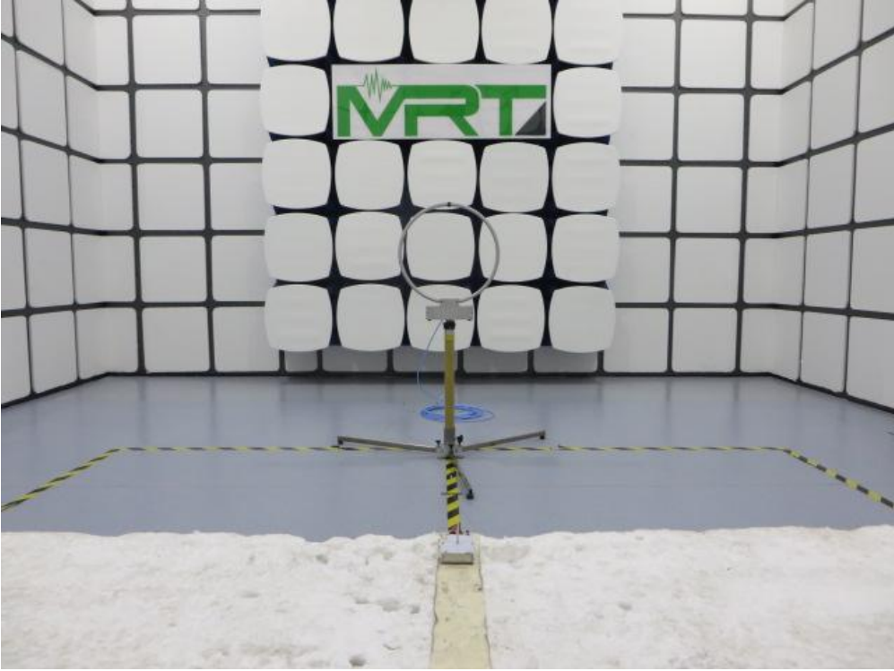
Description: Radiated Emissions Test Setup for Below 1GHz
