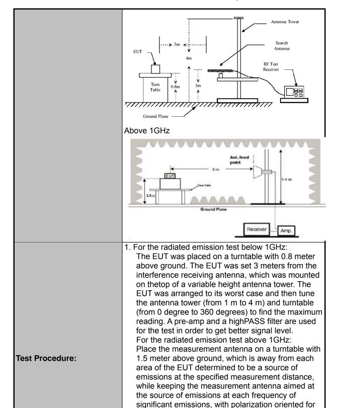
maximum response. The measurement antenna may have to be higher or lower than the EUT, depending on the radiation pattern of the emission
