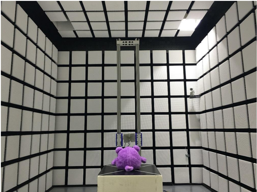
Spurious radiated emission for transmitter test above 1GHz
