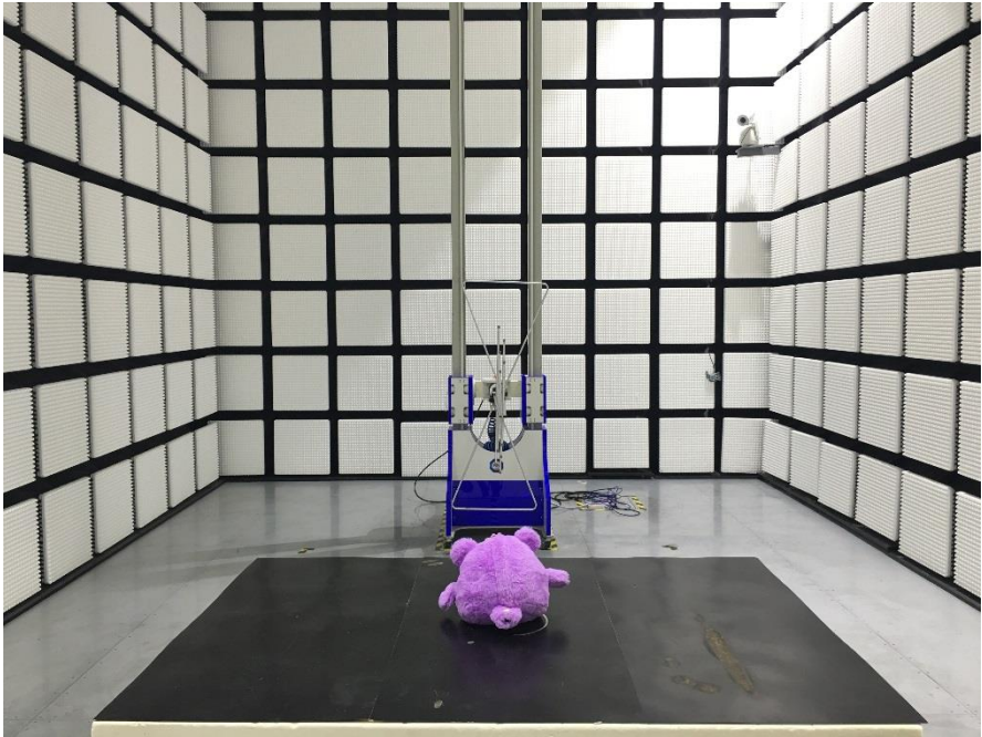
Spurious radiated emission for transmitter test above 1GHz
