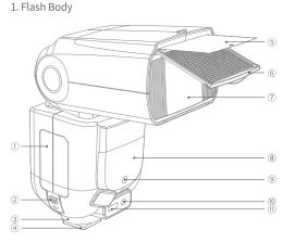
① Lithium Battery 2 Battery Eject Button 3 Hotshoe Attachment bracket
