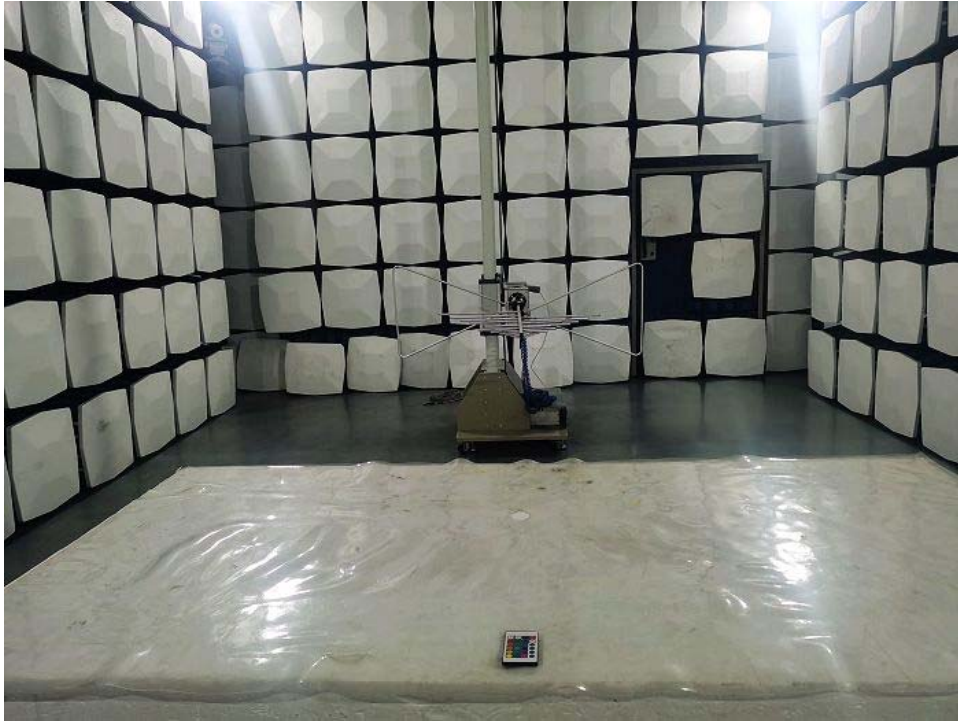
Radiated emission test view
