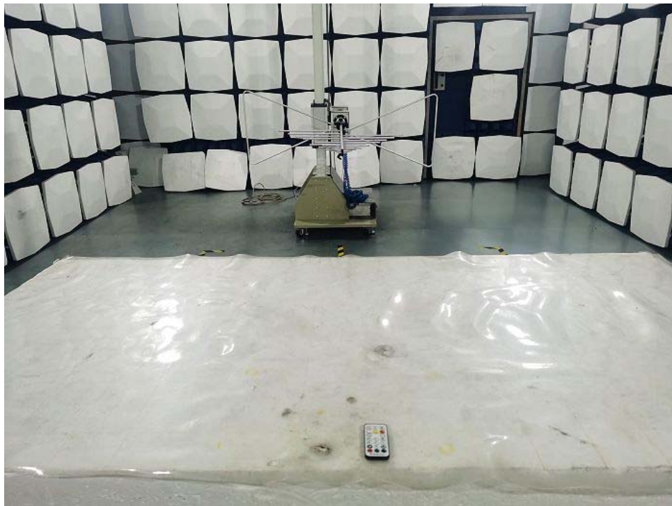
Radiated emission test view
