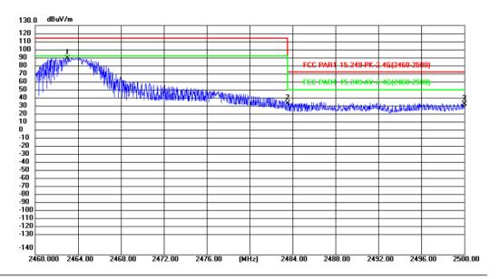
Site 966 chamber #1 Limit: FCC PART 15.249-PK-2.4G(2460-2500) Polarization: *Horizontal* Power: DC 3.0V
