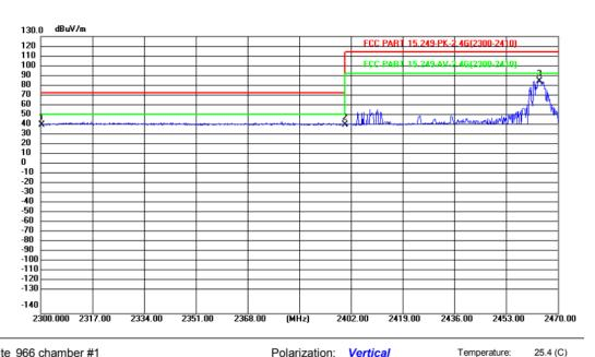
Site 966 chamber #1 Polarization: Vertical Temperature: Limit: FCC PART 15.249-PK-2.4G(2300-2410) DC 3.0V Humidity: Power:
