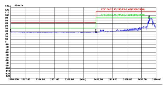
Site 966 chamber #1 Limit: FCC PART 15.249-PK-2.4G(2300-2410) Polarization: Horizontal DC 3.0V Power:
