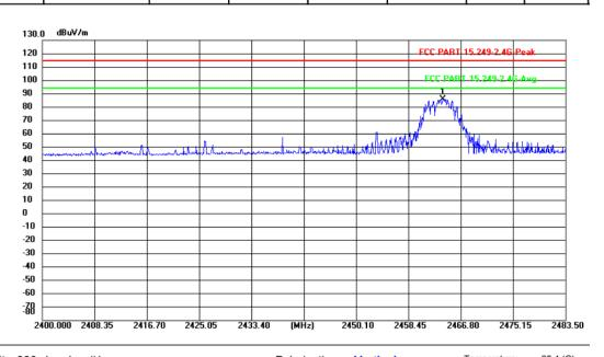
Temperature: 25.4 (C) Site 966 chamber #1 Polarization: Vertical Limit: FCC PART 15.249-2.4G-Peak DC 3.0V Humidity: 53.1 %RH Power: Reading Factor Limit Frequency Level Margin No. Detector (MHz) (dBuV) (dB/m) (dBuV/m)|(dBuV/m)(dB) 2463.961 -5.08 90.81 85.73 114.00 -28.27peak
