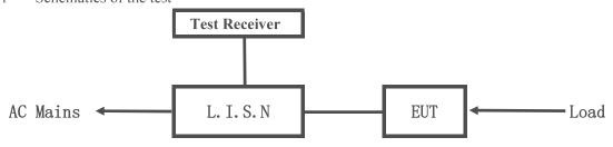
EUT: Equipment Under Test
