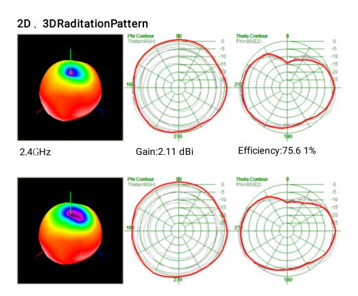
2.45GHz Gain: 2.23dBi Efficiency: 78.45%
