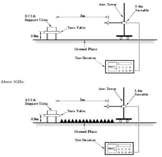
The radiated emission were performed in the 3 meters chamber test site, using the setup accordance with the ANSI C63.4-2014. The specification used was with the FCC Part 15 B Class B limits.
