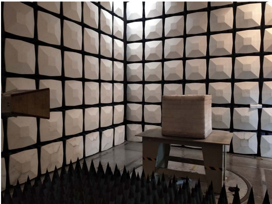
Radiated Emission Above 1GHz View
