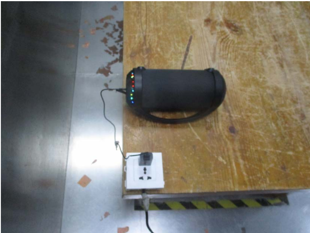
Conducted Emissions Side View
