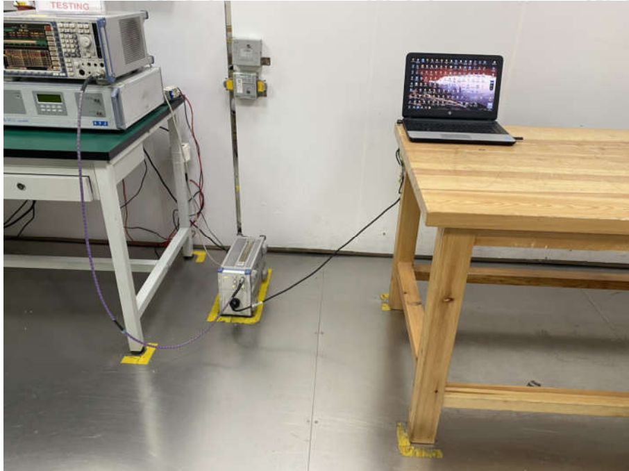
Conducted Emissions Test Setup-1
