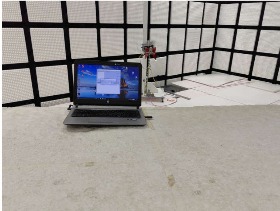
Radiated spurious emission Test Setup-3(Above 1GHz)
