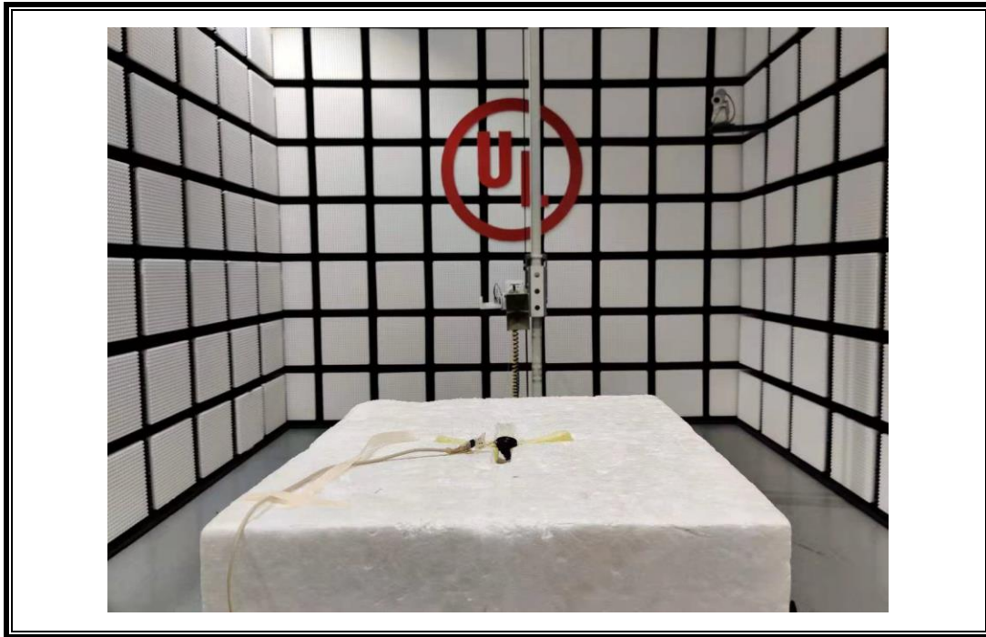
POWERLINE CONDUCTED EMISSIONS MEASUREMENT SETUP
