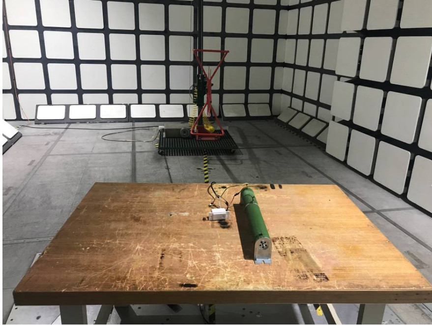
Radiated Emissions View (Below 1 GHz)
