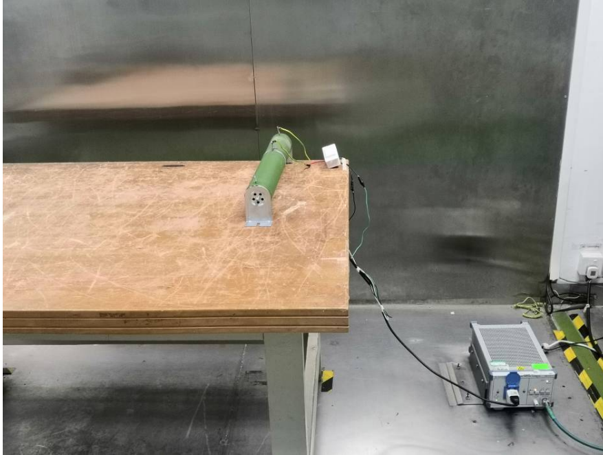
Conducted Emissions - Front View
