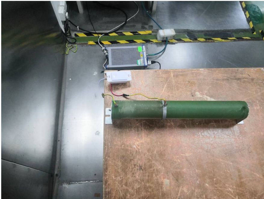
Conducted Emissions - Side View
