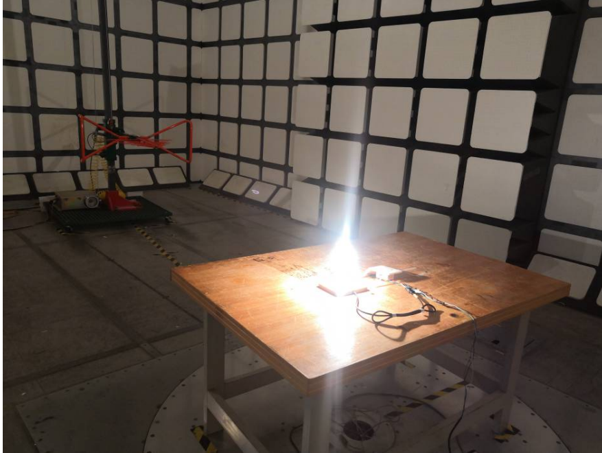
Radiated Emissions View (Below 1 GHz)
