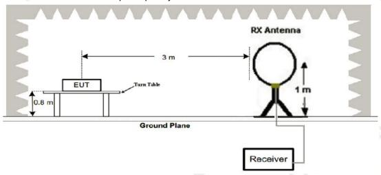
2. Radiated Emission Test-Up Frequency 30MHz~1GHz
