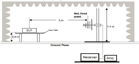
3. Radiated Emission Test-Up Frequency Above 1GHz
